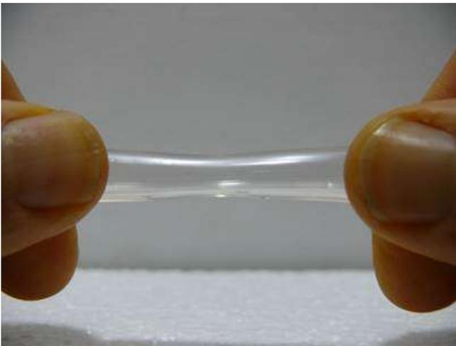
The same method works on the spout end. Here you heat the new tube approx. 2 inches from its end, heat the area, grab the (hopefully still cool) end, pull the tube apart and hold it for a few seconds till it's cooled off (you can hold the still hot stretched tube part in a stream of water, too, to speed cooling). The heated part will stretch and get thinner. Then cut the tube with your scissor at the thin part and push it into the spout opening with a bit of water for lubrication.
