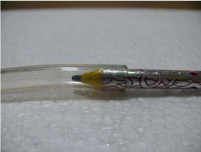
To get the tube onto the pump outlet, widen it by heating the tube material with the flame of a lighter (be sure not to burn it) and then pushing a pencil into the opening when the tube end is still hot and soft. It will then slip onto the pump easily.
